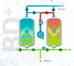
The blower (5) takes ambient air and blows it over the external heater (6). The heated air is then sent through the saturated desiccant (2), forcing the adsorbed moisture out, from top to bottom.
